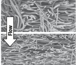
Figure 2. 3M™ DF Series Graded Porosity Media
