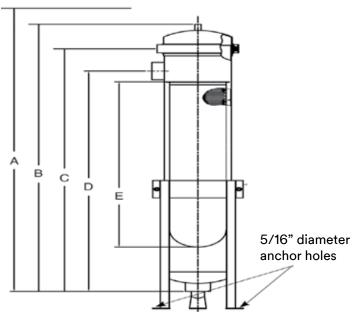
Leg Anchor Bolt circle is 10.5" (26.7 cm) diameter Legs are adjustable to a distance of 12" (30.4 cm)
