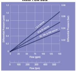
\* #2 Size Element and Support Basket Pressure Drop Only, housing pressure losses are not included.
