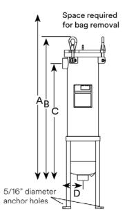
Leg Anchor Bolt circle is 10.5" (26.7 cm) diameter Legs are adjustable to a distance of 12" (30.4 cm)
