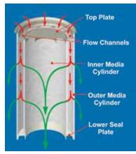
Figure 1. 3M™ DF Series Flow Path
