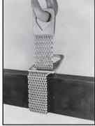
**NOTE:** The choker fitting must not be positioned against a load edge or directly on the triangle fitting.
